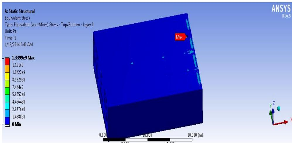
Maximum Equivalent Stress at mid ship 148 MPa
