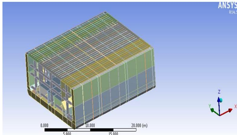
The length of each cargo hold is 6.6 m along the length of the vessel and 0.6 m empty space for separation of cargo are provided at the end of each cargo length.
