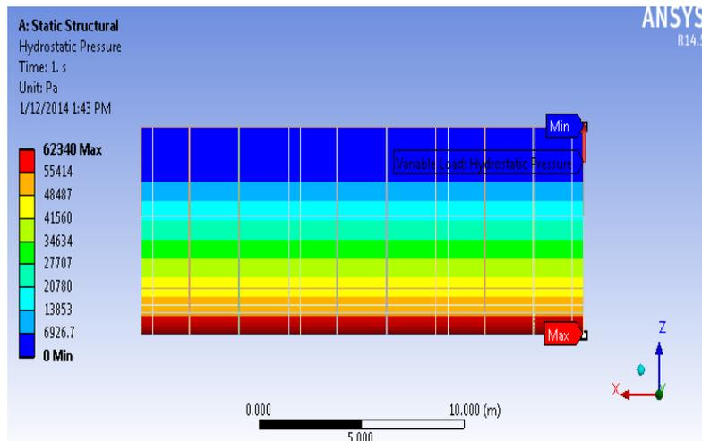
Maximum Hydrostatic Pressure = **62340 Pa**
